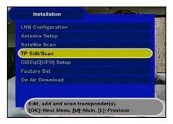
In this menu you can scan through the transponders for specific programmes, e.g. when new programmes are offered in the package of a specific broadcaster. You can obtain this information from SAT 1 teletext or corresponding TV and satellite magazines as well as from the Internet.
